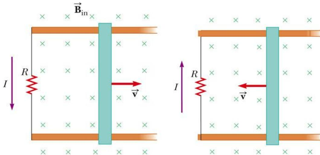
As the bar is slid to the right, the flux through the loop increases.
