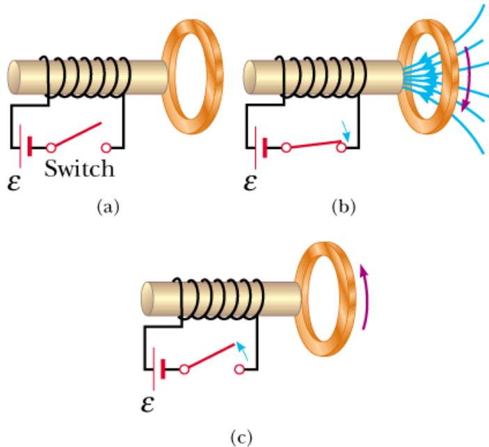
When the switch is closed, the flux goes from zero to a finite value in the direction shown.
