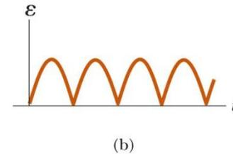
$$\Phi_B = BA \cos \theta = BA \cos \omega t \longrightarrow \mathcal{E} = -N \frac{d\Phi_B}{dt} = -NAB \frac{d}{dt} (\cos \omega t) = NAB \omega \sin \omega t$$
